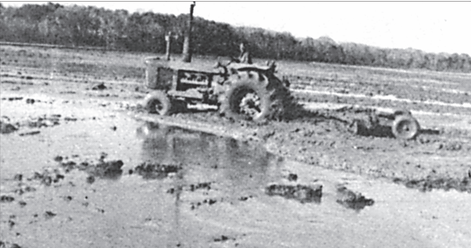
Water land leveling on Haidusek Bros. farm. Water leveling saves time, labor, fuel and machinery cost in growing rice.
